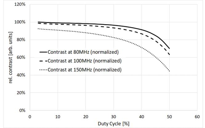
Fig. 9. Rel. contrast vs Duty Cycle for several modulation frequencies. Reduction of Duty Cycle permits higher contrast
