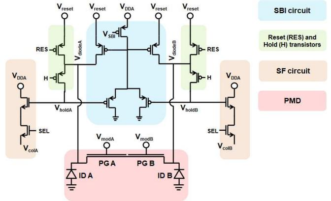
Fig. 2. Pixel schematic for  $7\mu\text{m}$  pixel
