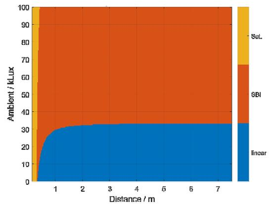
Fig. 4. Expansion of pixel operating range in background light with SBI (simulated: 1W 940nm VCSEL, 50nm optical filter,  $F\# 1.58$ ,  $500\mu\text{s}$   $T_{int}$ , 90% target reflectivity)
