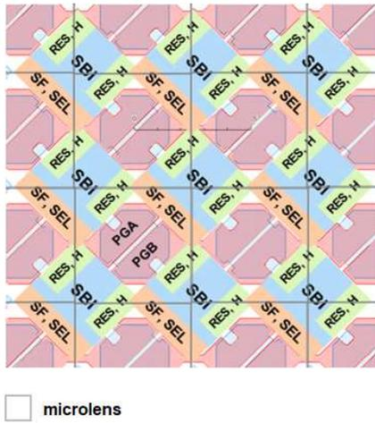
Fig. 5. Layout of rotated 5µm pixel
