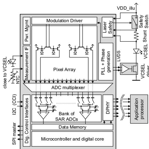
Fig. 6. Top level sensor architecture
