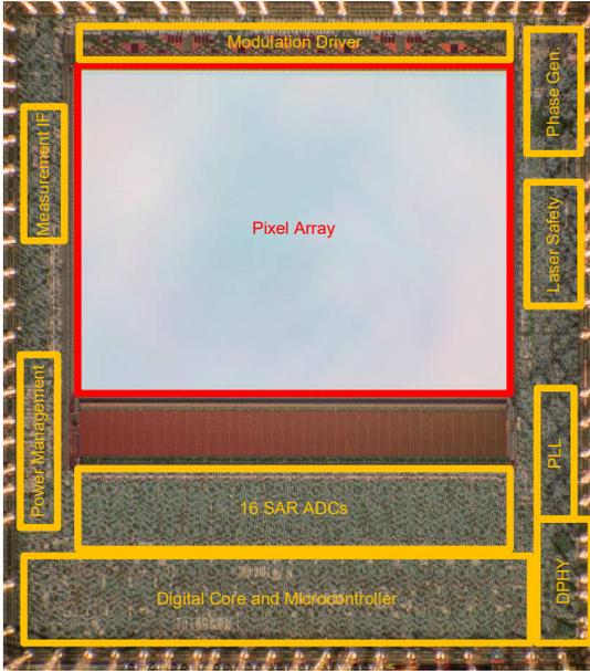
Fig. 8. Chip Micrograph of sensor with 153k  $7\mu\text{m}$  pixels
