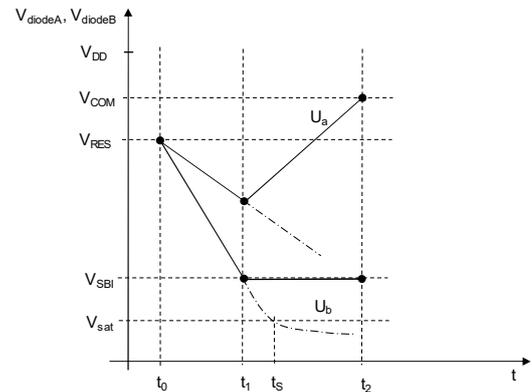
Fig. 3. Working principle SBI: channel B with higher signal from photocurrent reaches  $V_{SBI}$  threshold first. Saturation is avoided by a compensation current in channel A and B.
