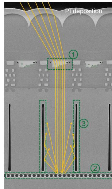
Fig. 1. Pixel cross section showing (1) prism, (2) mirror, and (3) deep trench
